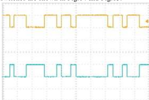
Fig.14 Gate pulses for switch 5 & 8
